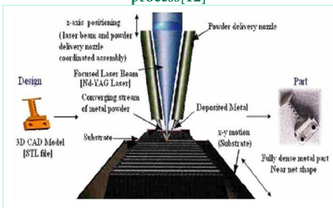
Fig. 1.1 : A schematic diagram of the LENS process[12]
