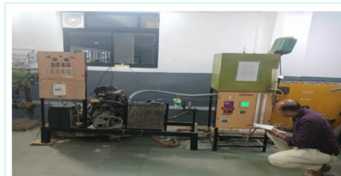
Experimental set up four strokes four cylinder 1.1 ltr. Petrol engine test rig
